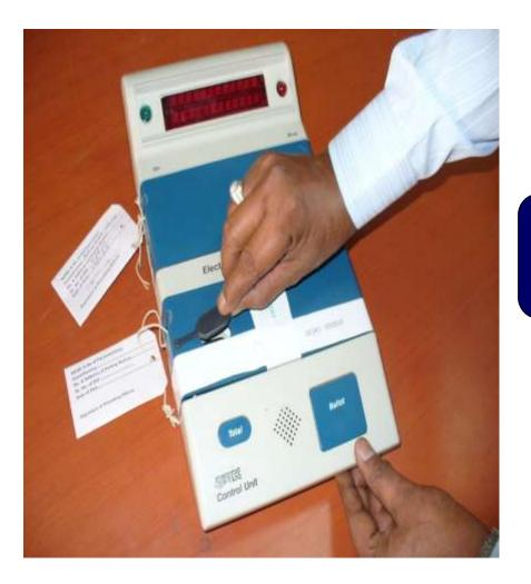
After the Close of POLL, remove the cap on Close button in the Control Unit.
