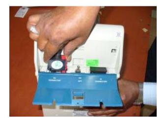
Open the bottom compartment of the Control Unit and Switch OFF Power and disconnect the interconnecting cable
