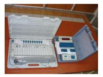
Pack the Control unit (with the Strip seal) and Balloting Unit in their carrying cases
