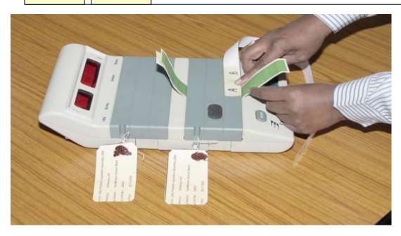
Keep the Strip Seal with pre-gummed portion 'A' near the base of the Green Paper Seal protruding from the lower end of the door.
