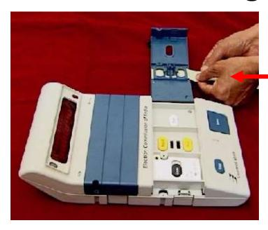
Insert the Green Paper seal in the frames provided for both Result
