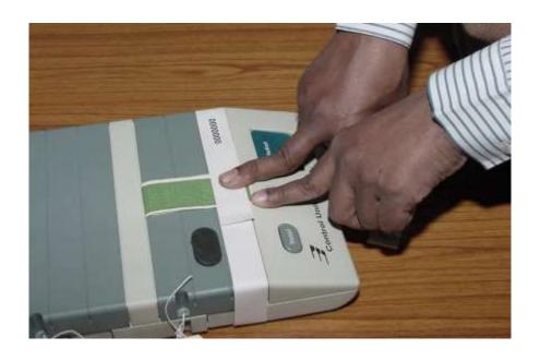
Now the Strip Seal is finally fixed. Note that the Strip seal does not cover CLOSE button Flap. Control Unit is now ready to take real poll.
