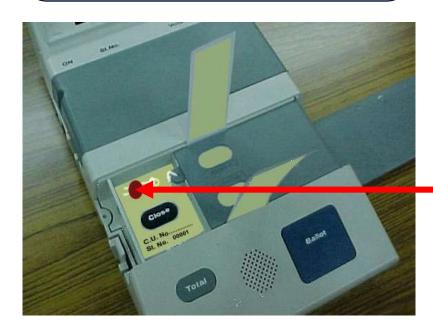
Fix the Special tag such that the Close button is visible and seal the tag
