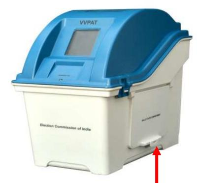
The Pr. O and polling agents shall put their signatures on the address tag for sealing of Drop box of VVPAT after completion of mock poll. (51/8/VVPAT- INST/2019-EMPS dt. 15.11.19)
