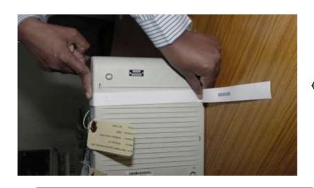
Take the Strip Seal round the Control Unit from left side just below the CLOSE button window
